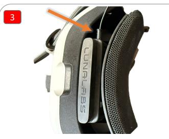
Plug the forehead electrode lead (arrow) into the side of the Electra.
