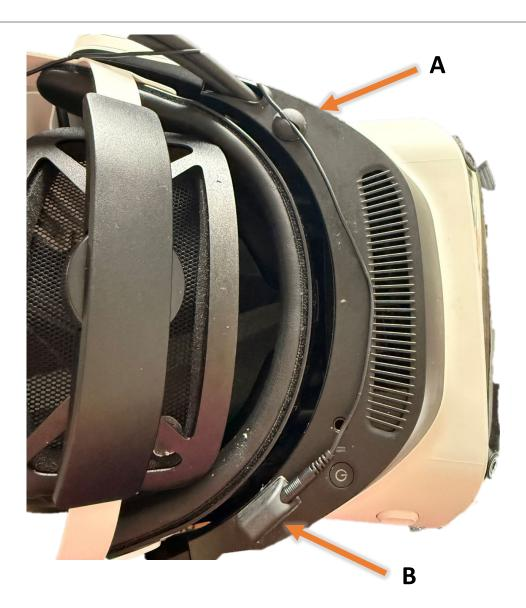
Remove the adhesive covers on the Cable Guide (A) and Wire Receptacle (B). Adhere them on headset as shown to secure front electrode lead.
