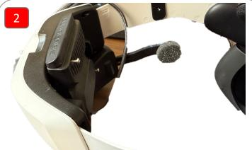
Align the 3WAVES Electra unit with three mounting holes in the rear of the headset. Use the provided screws to secure it into place.
